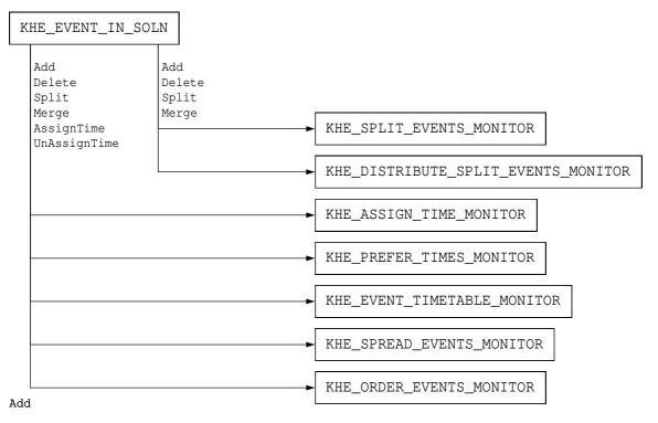
Split events and distribute split events monitors do not need to know about time assignment and unassignment. Based on the calls they receive, they keep track of meet durations and report cost accordingly. Assign time and prefer times monitors are even simpler; they report cost depending on whether the meets reported to them are assigned times or not.
