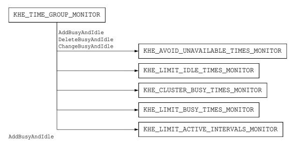
When a monitor is attached, function AddBusyAndIdle is called instead, and when a monitor is detached, function DeleteBusyAndIdle is called instead.
