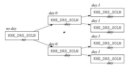
The day indexes in this diagram are open day indexes, not frame indexes. The search tree has one level of solutions for each open day, plus the extra level holding the root solution. The root solution is special in that, despite being a day solution, it has no day. There may be closed days, obviously, but they are not visible in the search tree.
