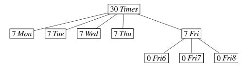
A postorder traversal of this tree may be used to deduce that workload demand nodes for r are needed for one Mon time, one Tue time, one Wed time, one Thu time, one  $Fri\delta$  time, one  $Fri\delta$  time, and three arbitrary times. In general, each tree node contributes a number of demand nodes equal to the size of its set of times minus its number minus the number of demand nodes contributed by its descendants, or none if this number is negative.
